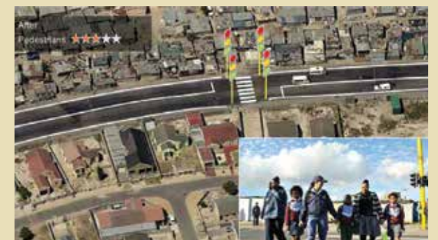
After: a new lights controlled crossing and traffic calming is estimated to have reduced risk by up to 80%
