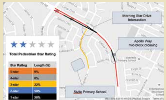
iRAP road assessment map showing star rating of local roads at the Sivile pilot site
